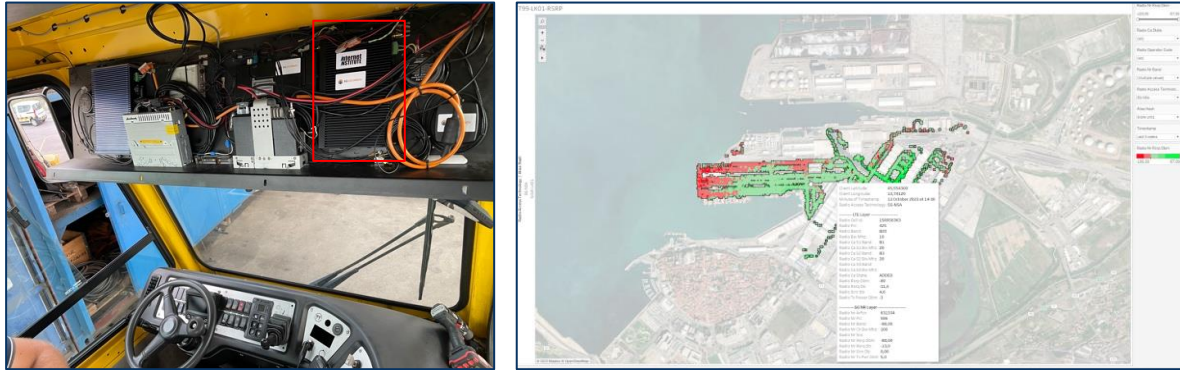
Figure 116: LL Koper - 5G IoT Gateway deployment on Terberg truck (figure on the left) used for drive testing and 5G performance analytics in the port (figure on the right).
