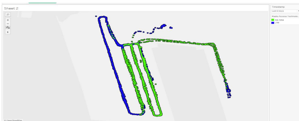
Figure 5: LL Athens - 5G drive test routes at Piers II and III, showcasing 5G and 4G coverage
