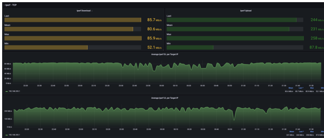
Figure 129: LL Koper - Private 5G SA - Throughput test results using 50 MHz NR BW (K-KP114)
