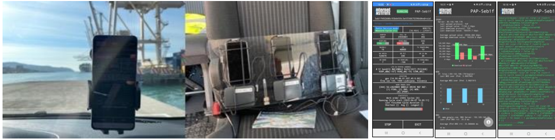
Figure 88: LL Koper - Drive test setup using qMON system on commercial smart phones.
