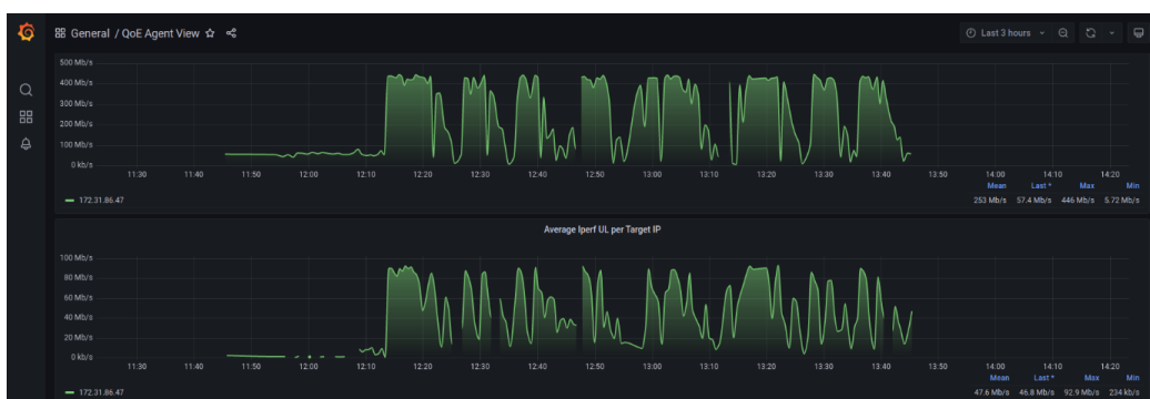
Figure 8: LL Athens - 5G drive test downlink and uplink measurements in 1.5 hours driving – (A-KPI20)
