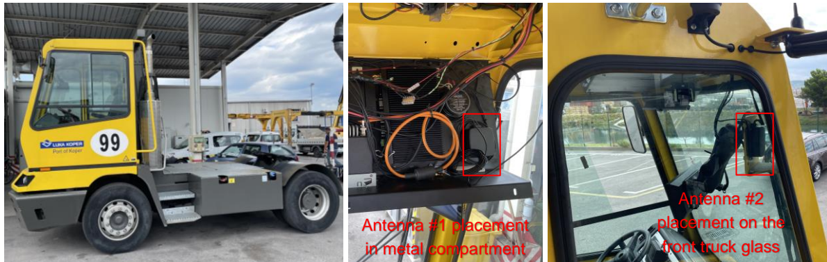
Figure 93: LL Koper - Yard truck equipped with ININ's 5G GW and qMON agent (left), placement of the 5G GW antennas (middle and right).
