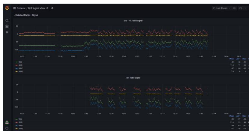
Figure 11: LL Athens - 5G drive test radio signal measurements (RSSI, SINR, RSRP, RSRQ)
