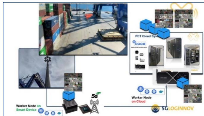
Figure 33: LL Athens - Components/installations of the 5G&AI enabled human presence detection use case
