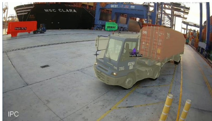
Figure 31: LL Athens - Inferred (segmented) video streams delivered to 5G handheld devices or central monitoring platform.
