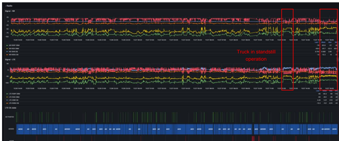
Figure 96: LL Koper – 5G drive testing with yard trucks showcasing 5G NR (NSA) performance variation on a time graph.
