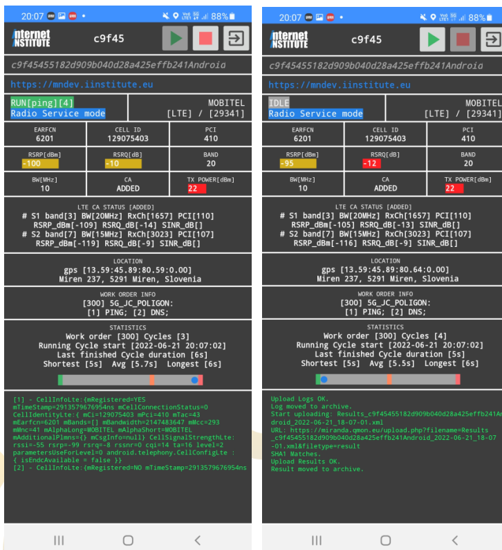
Figure 132: Screenshots showing qMON agent status (qMON agent is an Android application installed on the UE used for the test).
