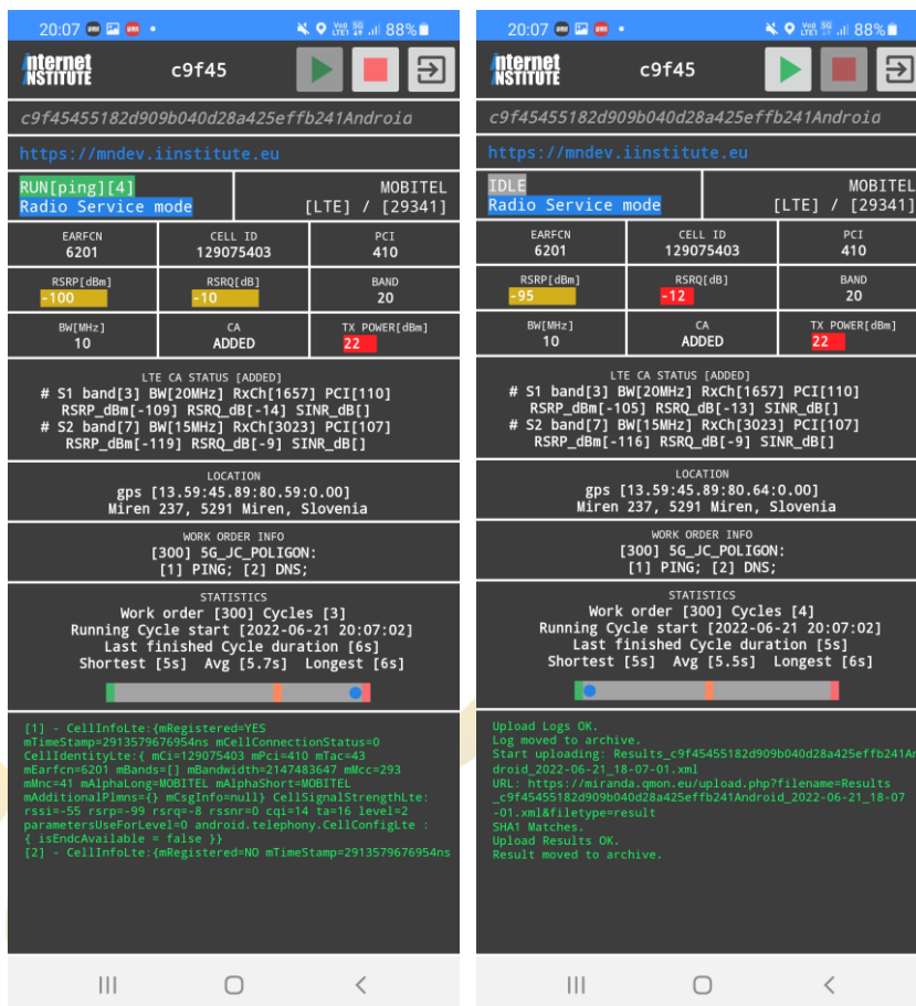
Figure 138: Screenshots showing qMON agent status (qMON agent is an Android application installed on the UE used for the test).
