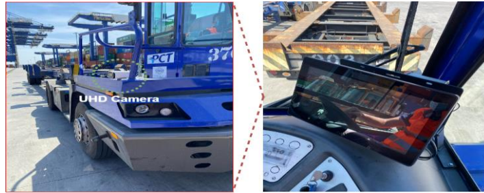
Figure 16: 4K camera and tablet installed on PCT's yard truck
