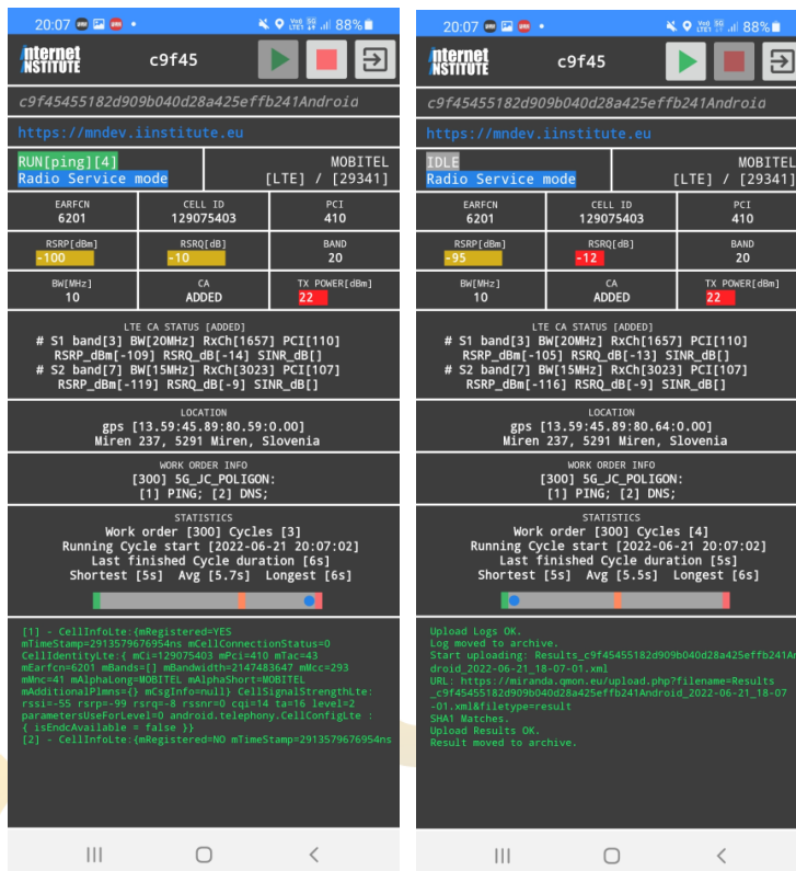
Figure 126: Screenshots showing qMON agent status (qMON agent is an Android application installed on the mobile device, i.e., smart-phone, used for the test).
