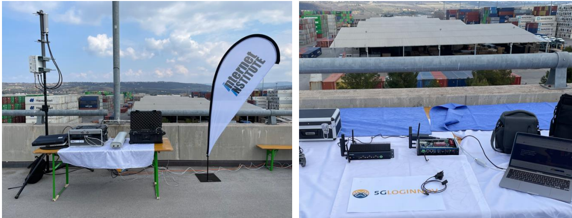
Figure 88: LL Koper - Private 5G SA system / 5G NR with 5G CN (left), 5G IoT GW (right).
