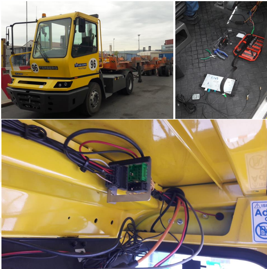
Figure 98 LL Koper - Installing Telemetry IoT Device in Port Terminal Trucks
