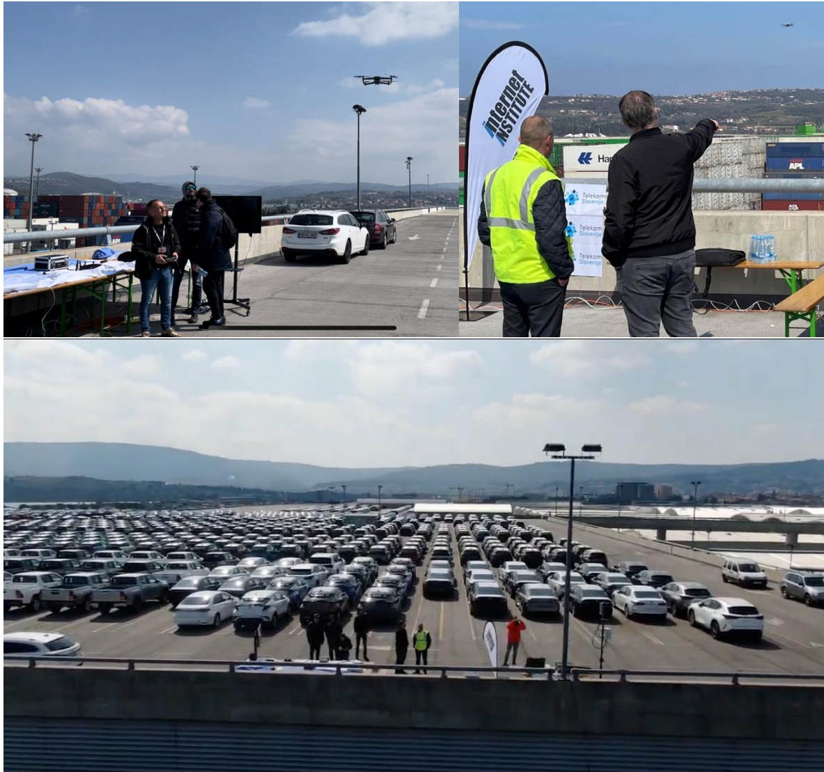
Figure 112: LL Koper - UC6 drone surveillance with RT-video streaming over the 5G SA network.
