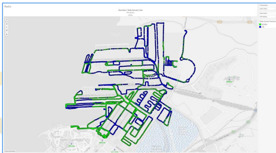
Figure 92: LL Koper - qMON Insight Analytics / 5G Drive testing in Koper LL / 4G vs 5G coverage results.
