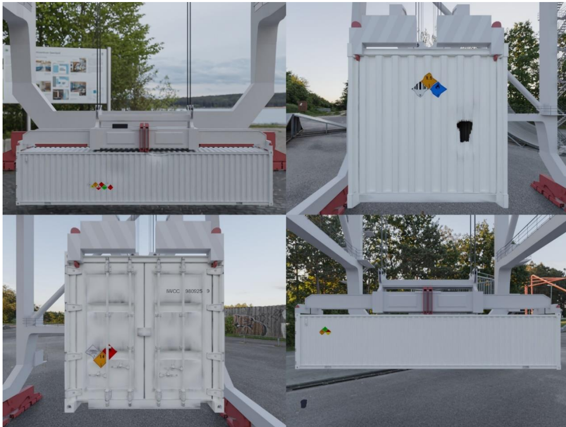
Figure 106: Koper LL - Synthetic data from the 4 cameras perspectives.
