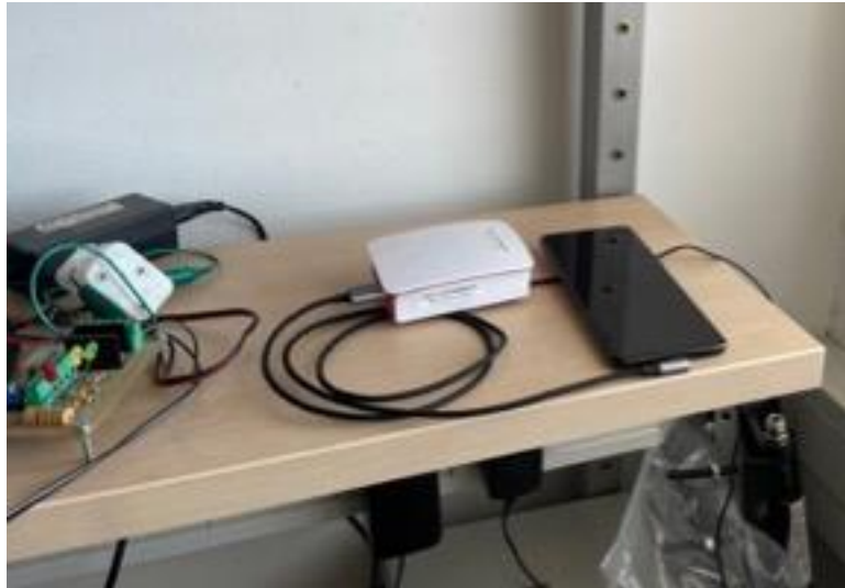
Figure 93: LL Koper - qMON Android Agent deployed in Koper LL as stationary test unit used for continuous 5G network and services monitoring.
