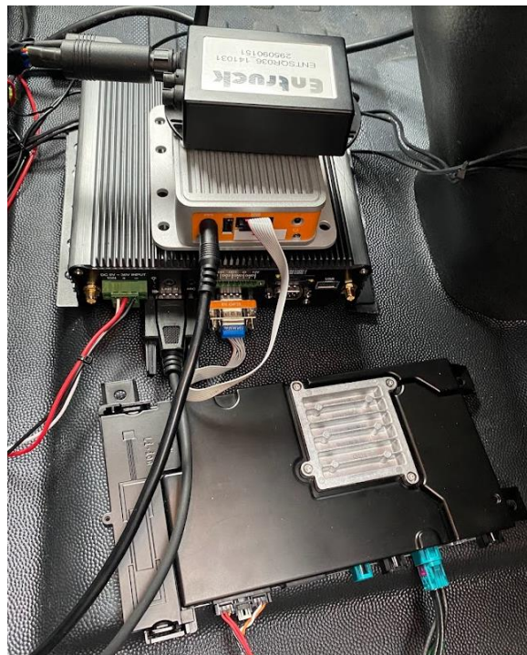
Figure 55: Entruck and Conti IoT devices installed in LL Hamburg
