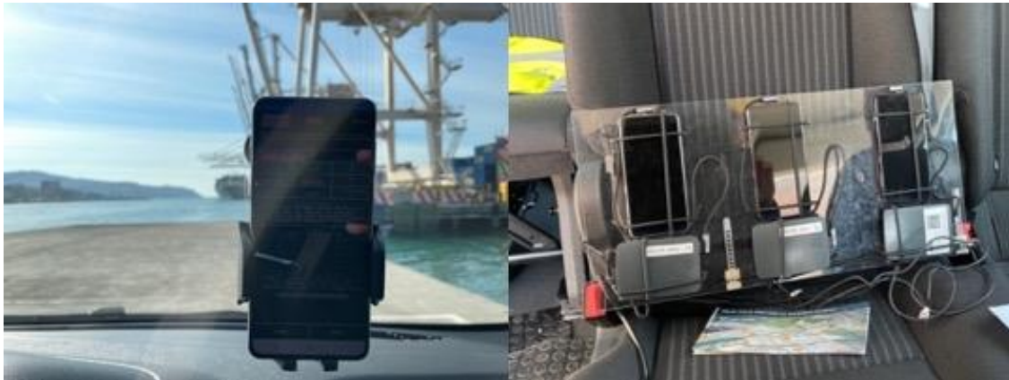
Figure 91: LL Koper - qMON Android Agents deployed in a vehicle as part of 5G network drive test in Koper LL.
