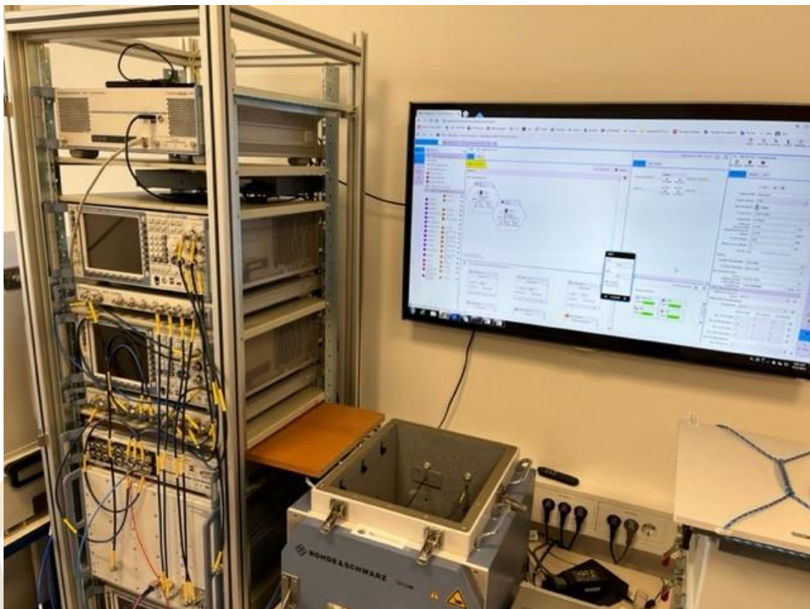
Figure 101: LL Koper - Test setup in Telekom Slovenije, for the Telemetry IoT device.
