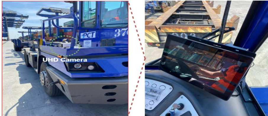
Figure 21: LL Athens UHD Camera installation on PCT's Yard truck.
