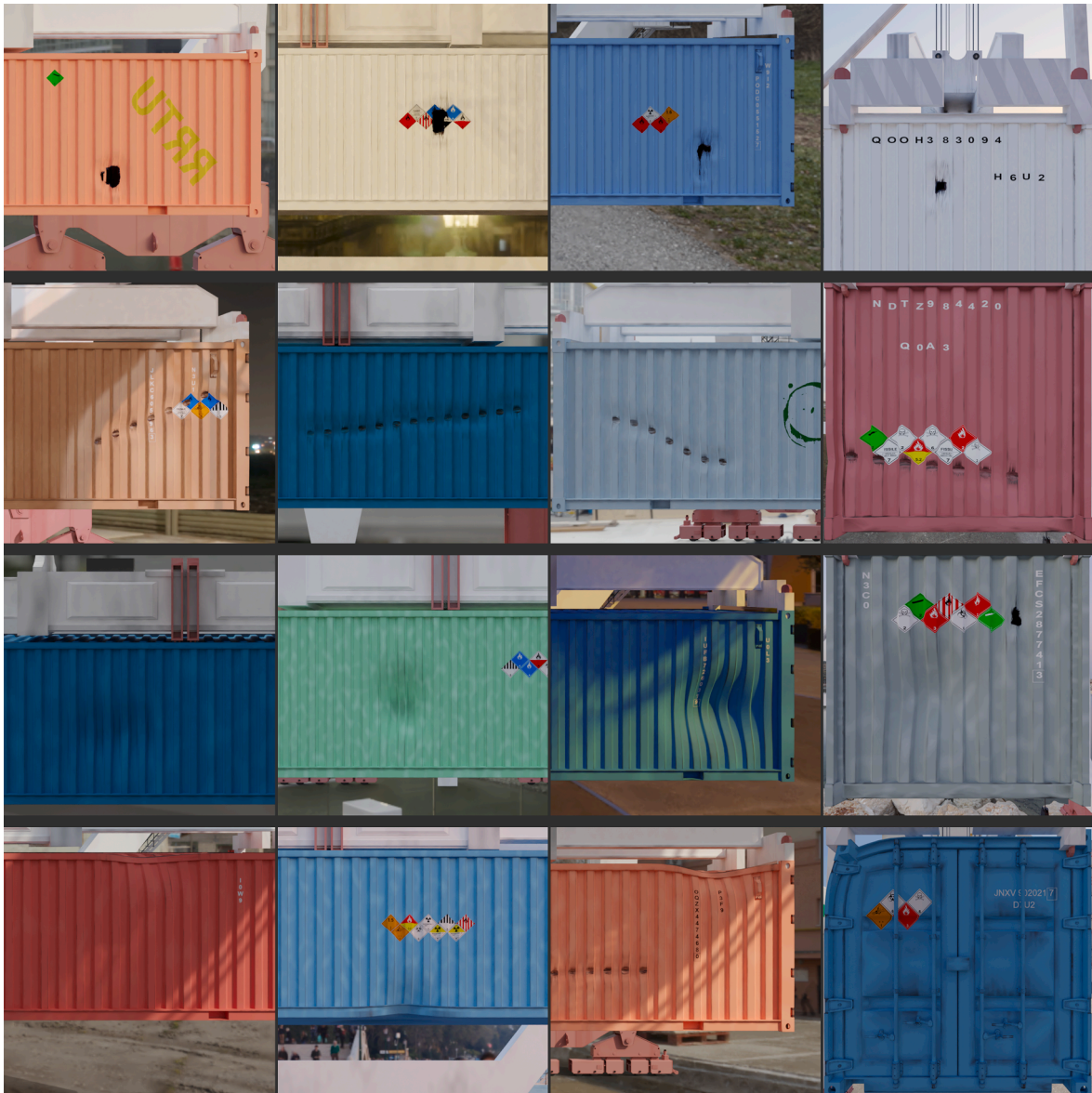
Fig. 2. Different types of damages that are generated. From top to bottom we find perforation, dented, concave and axis.
