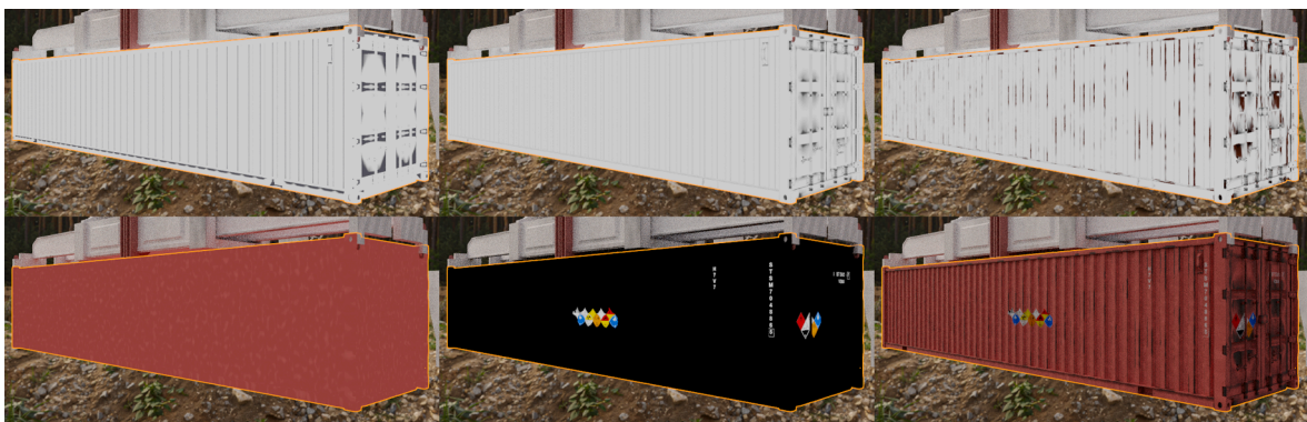
Fig. 5. Achieving realistic container representation through material compositing. Top row: Aging, dirt, and rust effects. Bottom row: Tone variation, IMDG markers, and reflections.
