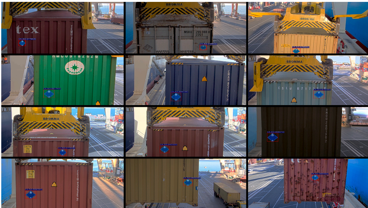
Fig. 12. Results of real images in order to test the domain gap for the detection of container and text classes marked with green and red colours respectively.
