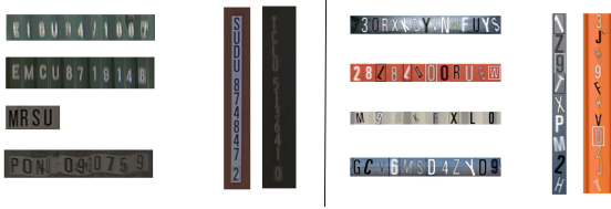
Figure 3: Detection patches from real images (left). Synthetic character sequence generated image (right).
