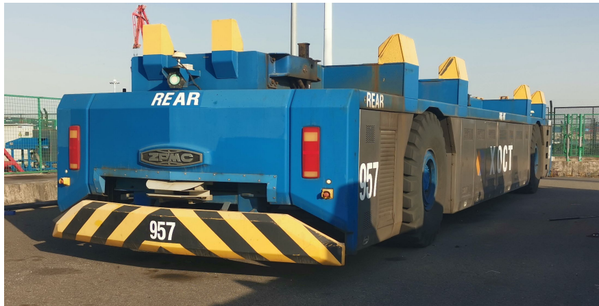
Unmanned IGV: 5 cameras (3 front + 1 rear + 1 full view)
