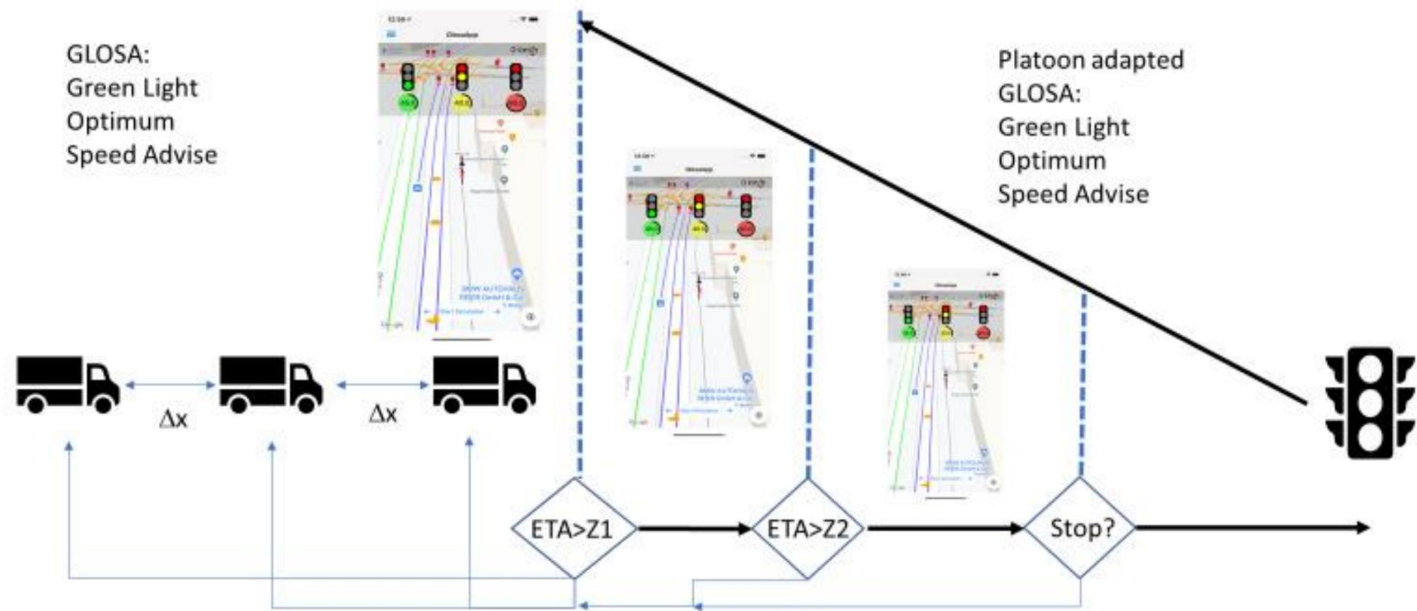
ETA: estimated time of arrival / Z: threshold trigger to stop Truck Platoon
