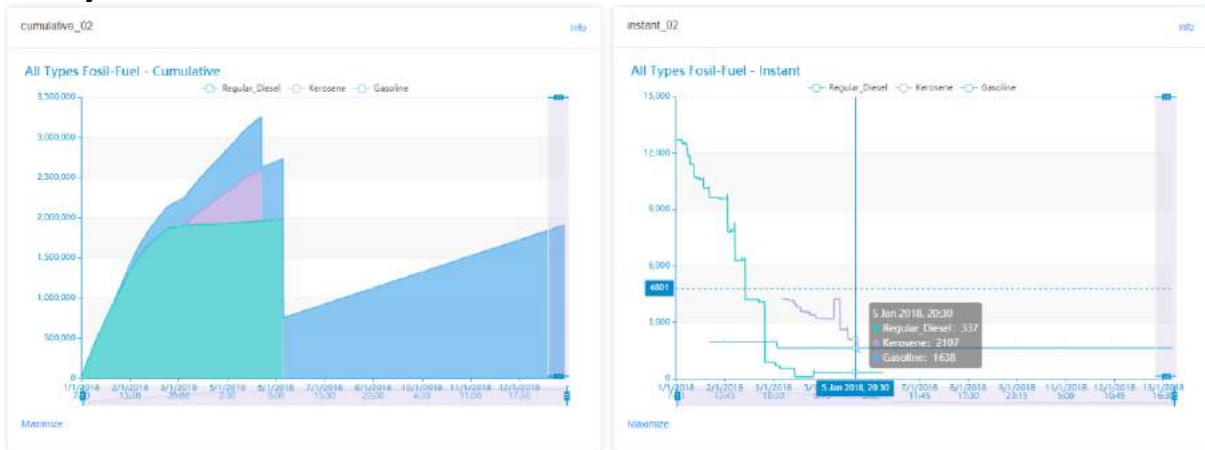
Figure 8: Example of results of the energy model (via the PIXEL platform GUI). Results can be filtered by energy type and be displayed as instant or cumulative consumption.
