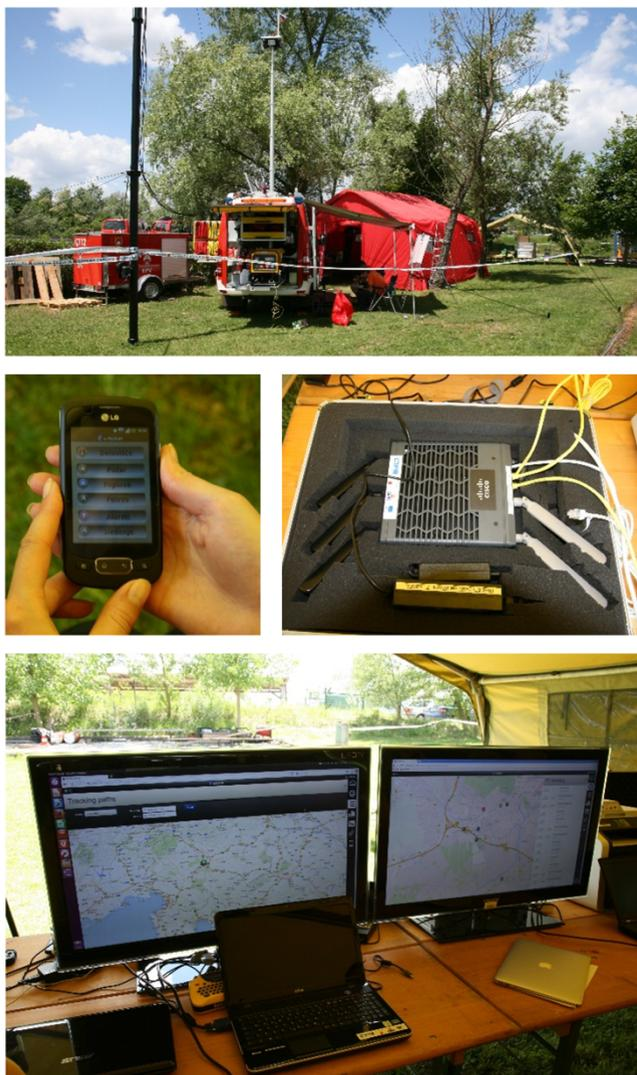
**FIGURE 19.** Field experimentation with the PPDRone facility and tools at the International Rescue Dog Exercise in Ljubljana, Slovenia. The figure displays the BoO with the tactical command vehicles and communications infrastructure (top), the mobile triage and tracking application installed on a ruggedized smartphone (middle left), the industrial IoT gateway (middle right), and the intervention monitoring dashboard set up at a workstation in a temporary BoO sheltering (bottom).
