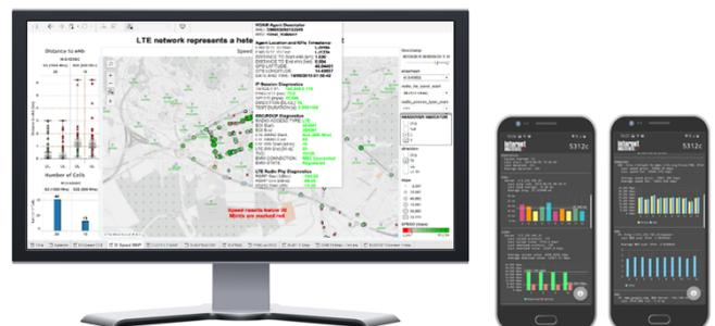
**FIGURE 8.** PPDR applications available in the PPDRone facility – a production-grade network and service testing, verification and benchmarking system with a dashboard (left) and mobile agent probes (right).
